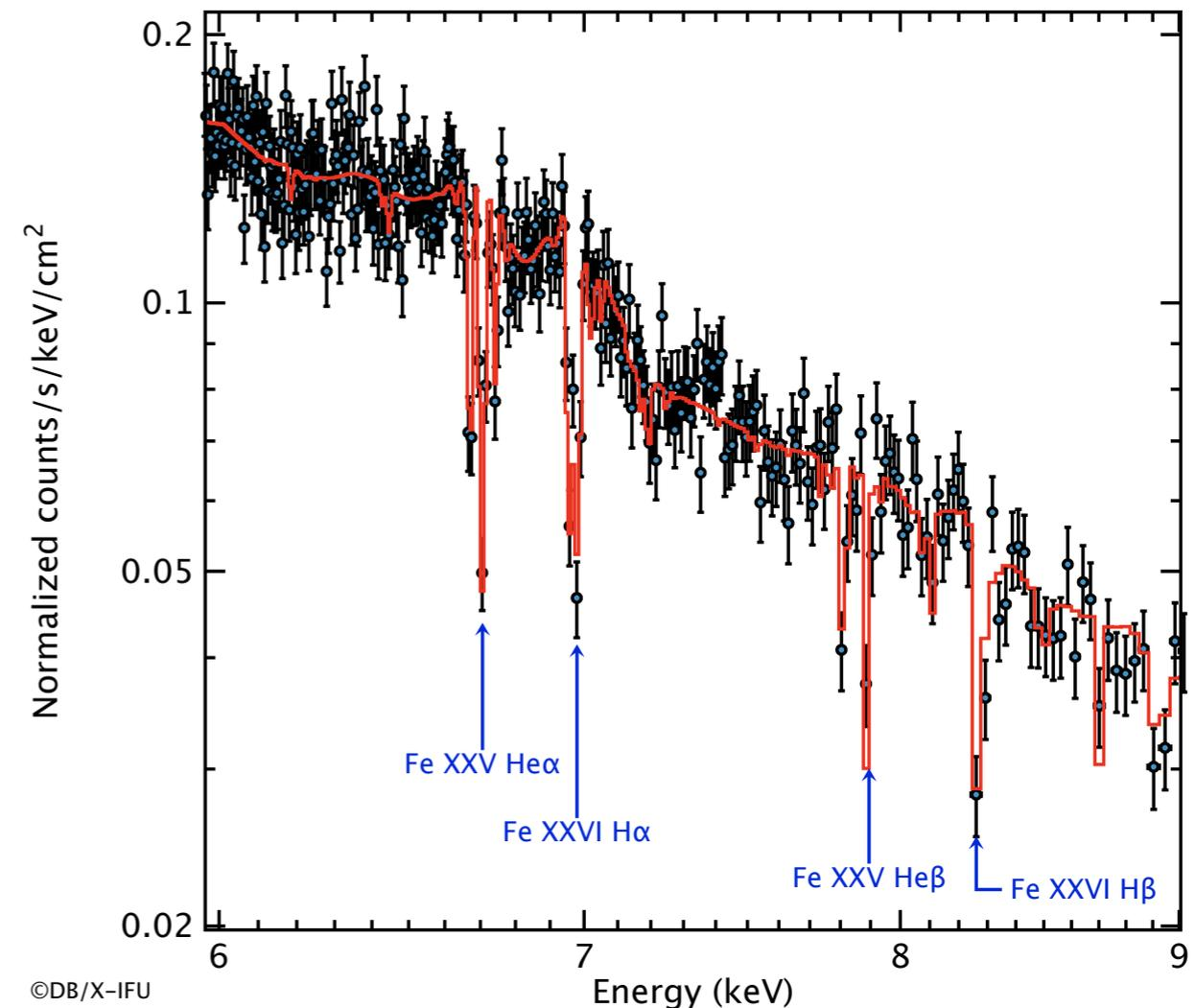
X-ray binary spectrum with high velocity wind absorption features. Courtesy of J. Miller et al.
