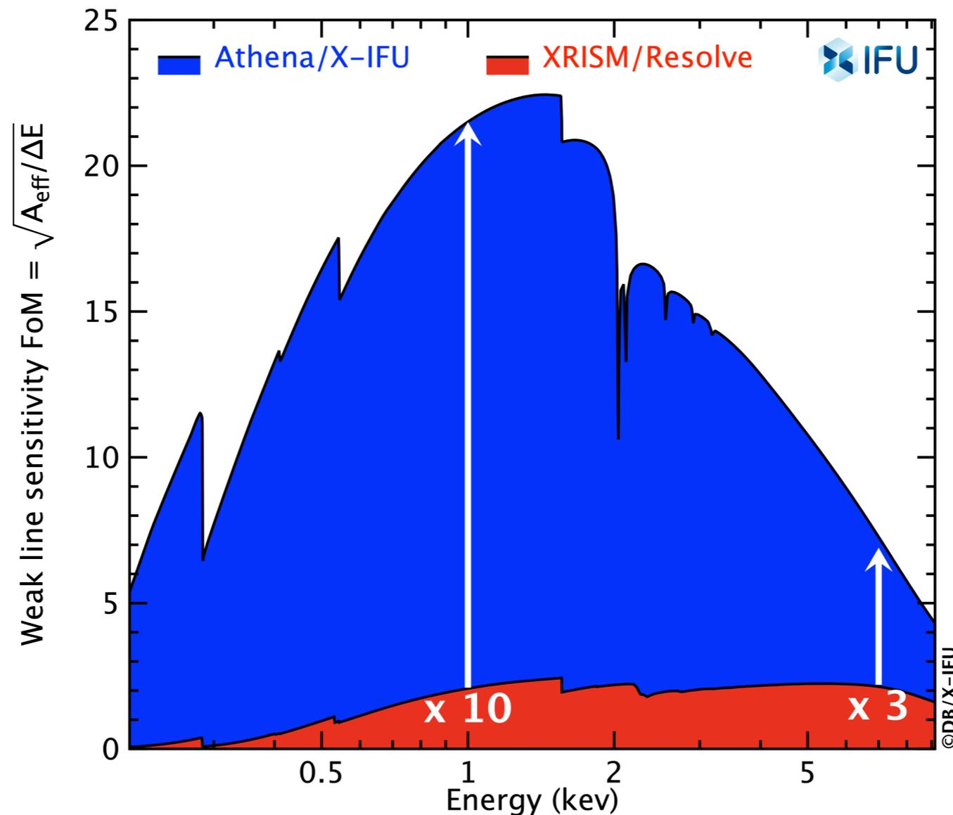
Comparison of the weak line sensitivity of Athena X-IFU and XRISM Resolve spectrometers
