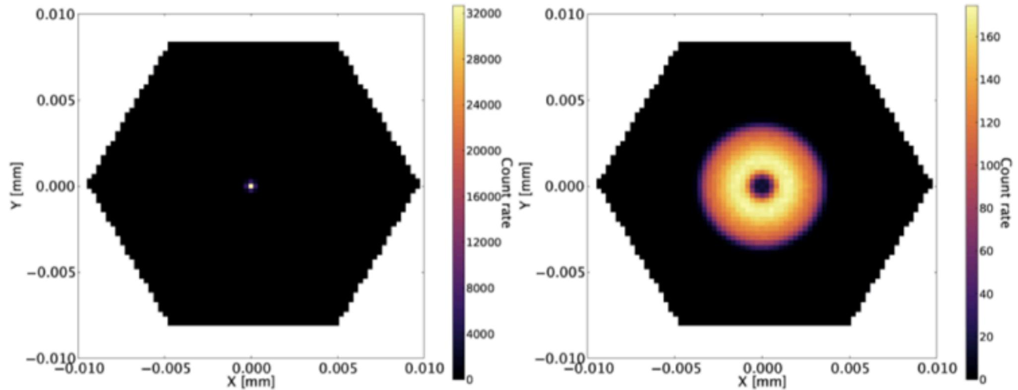
A point source in focus and out-of-focus by 35 mm
