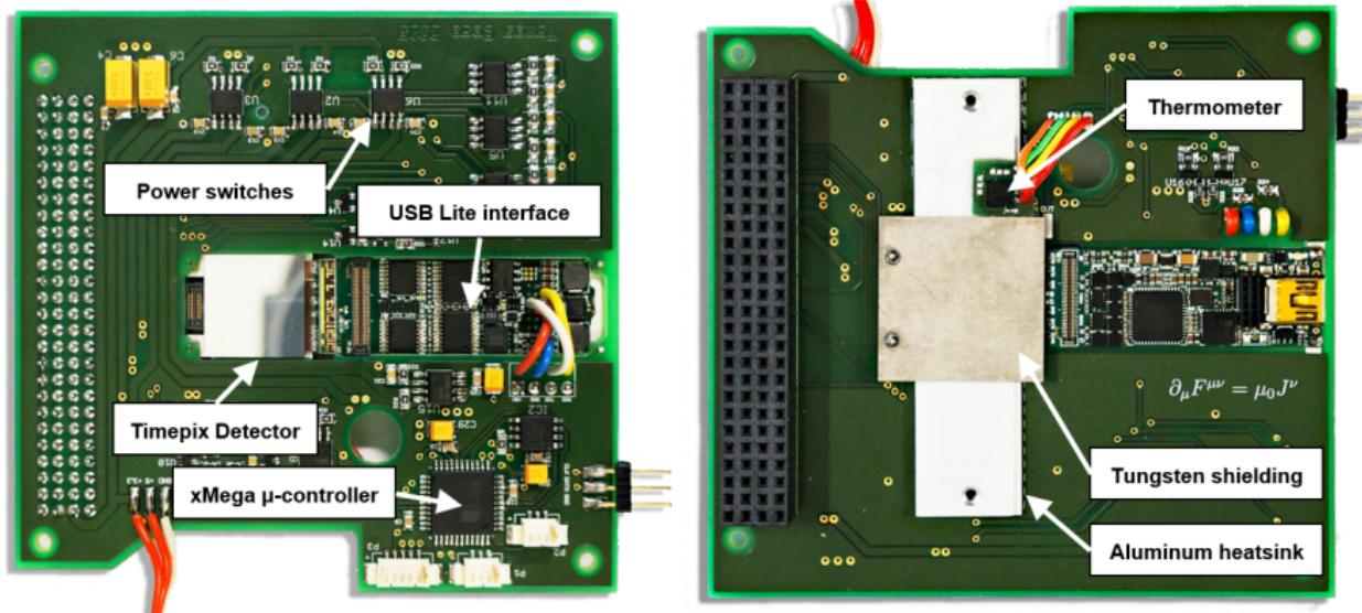
Figure: X-Ray sensor board
